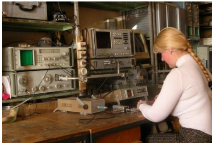
Fig. 3 Krasnoukhov V. N. (Mandrygina) at laboratory installation for measurement of dielectric permittivity of soils in the range of 0.1-17 GHz (2002).
