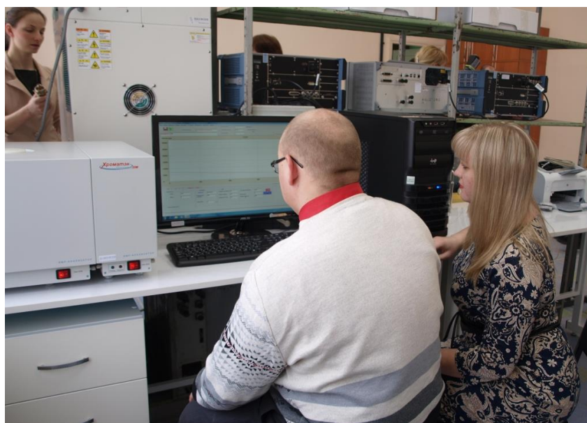
Fig. 8. Apparatus for investigation of rock petrophysical characteristics by nuclear magnetic resonance method (a Nuclear Magnetic Resonance Relaxmeter HROMATEK PROTON 20 M)
