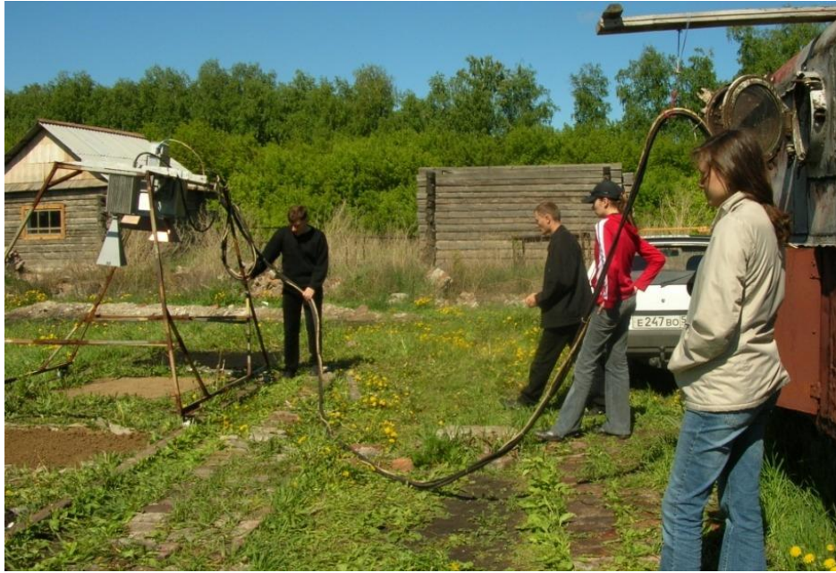
Fig. 2. The ground for a research of a radio –heat radiation of soils in a frequency range of 2.7-8.3 GHz (the agrostation OSPU of 2001-2005).
